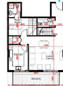
2 Bedroom Duplex Type 3 Apartment Area: 205.90m 2 (2,216.69ft 2 ) Suite Area: 176.60m 2 (1,902.27ft 2 ) Balcony Area: 29.30m 2 (314.01ft 2 )
